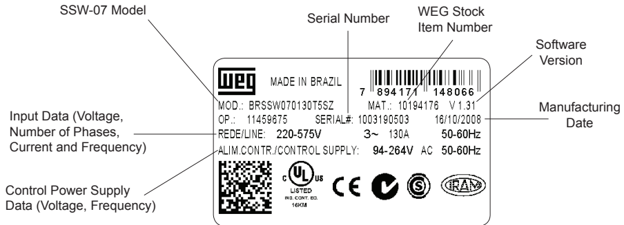
Figure 2.3 - Soft-Starter SSW-07 identification plate
